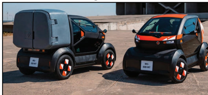
Two versions of the Mobilize Duo, consumer and commercial. These are classified as heavy quadricycles or L7es in the European quadricycle definitions. There is nothing comparable in the U.S. based NHTSA vehicle classifications.
