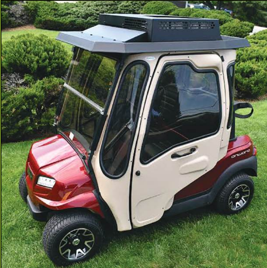
PHOTO: Fully enclosed golf cart with an integrated cabin AC system. Source: Curtis Cabs
